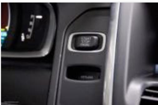
APPUYEZ UNE FOIS SUR LE BOUTON DE DÉMARRAGE ET D'ARRÊT POUR METTRE LE SYSTÈME SOUS TENSION.
